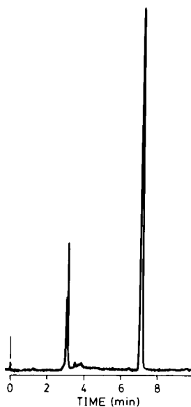
Fig. 4. Chromatogram of flow-cell performance test mixture. Components: acetone, 1%; sodium chloride, 250 ng/ml; pyrene, 1000 ng/ml in acetonitrile-water (65:35). Mobile phase, 100% acetonitrile.
